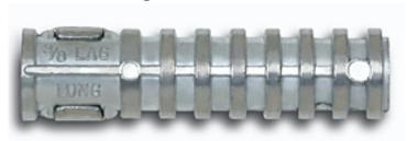
The lag shield is a screw style anchor designed for use with lag bolts. Lag shields are suitable for use in concrete and the mortar joints of block or brick walls. In harder masonry materials, short style lag shields are used to reduce drilling time. The long style lag shield is used in soft or weak masonry to better develop strength. The lag shield is not recommended for overhead applications.
